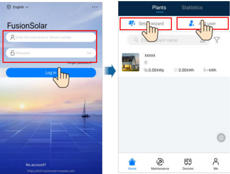
Figure 7-3 Creating a plant and an owner account
